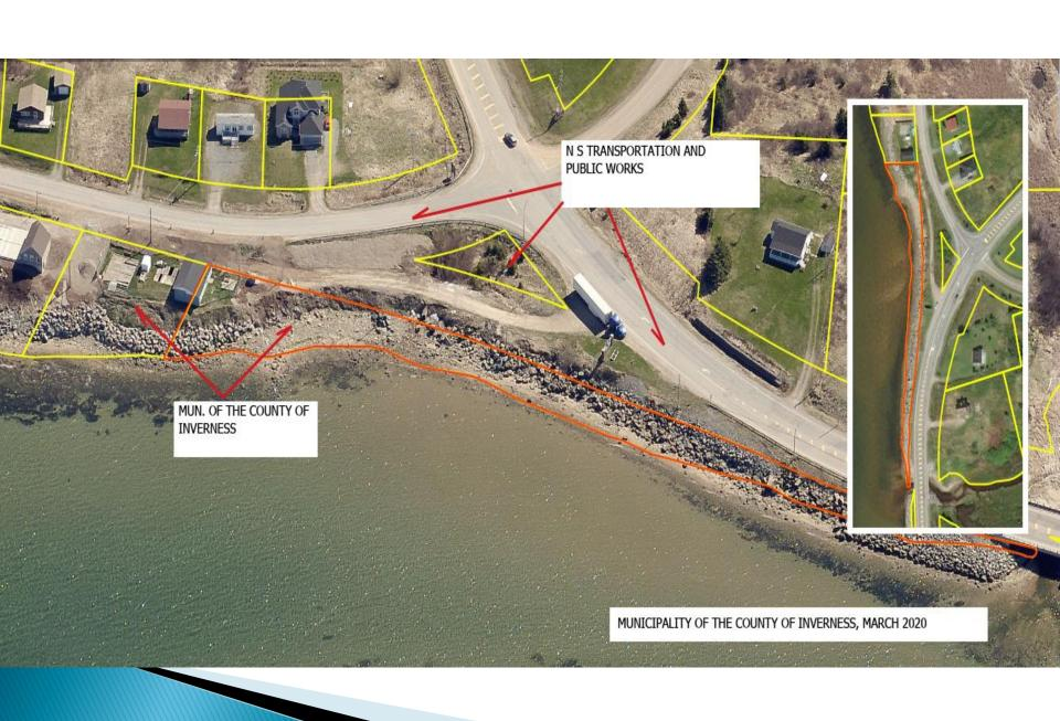
In 2019 some work was completed on the section owned by DTIR. Thirty inch pipe was put in to connect to the existing culvert under Main Street and connected to manhole.
